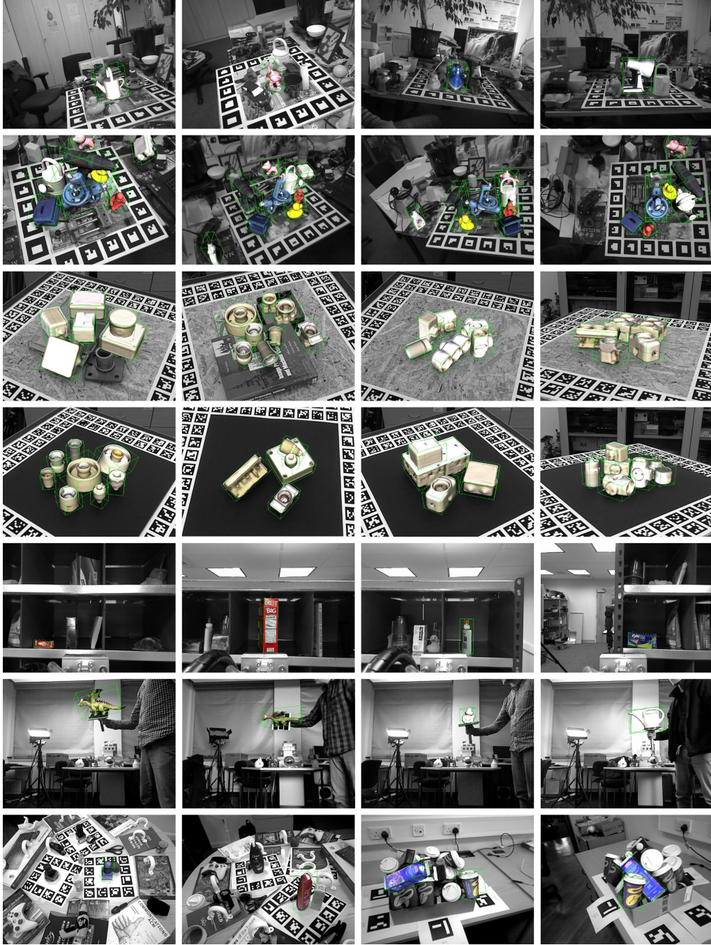
Figure 5.7: Proposed method results in scenes from the BOP benchmark datasets. Scene RGB data is shown in gray. Object models are shown in color and inside a green bounding box. Notice that, for scenes with multiple instances, only the most supported instance is used.
