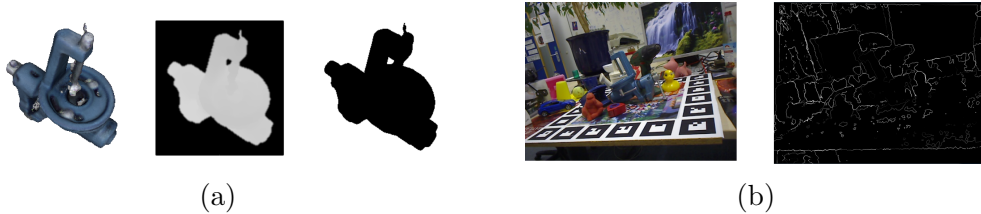
Figure 3.5: Examples of the extraction of the object model silhouette and the scene edges. (a) object model silhouette; (b) scene edges.
